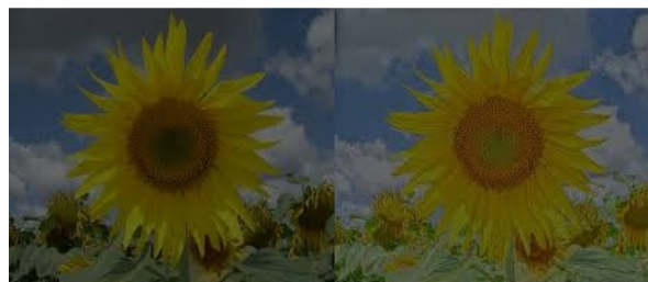
Fig.1 An image displayed on an LCD with (a) 10 % backlight and (b) 100 % backlight.
