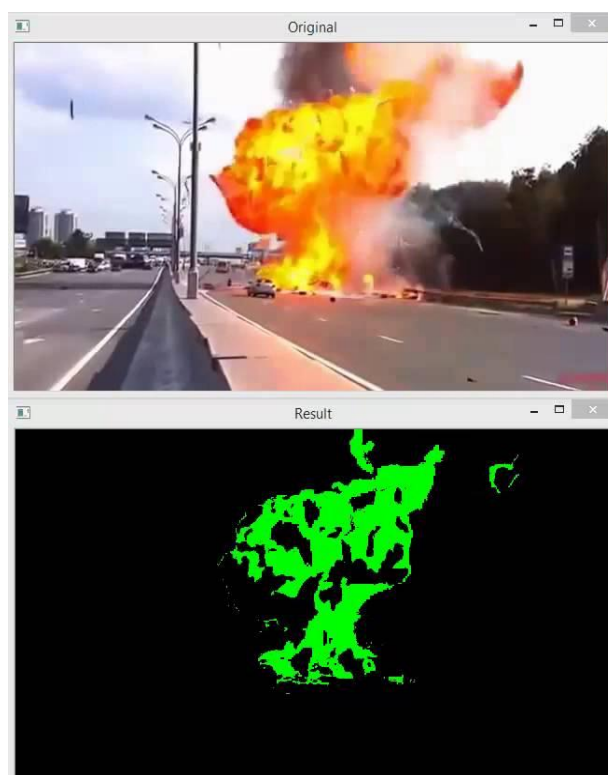
Figure 2. Image Processing based Fire Detection [2]
