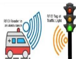
Figure 1. Ambulance and traffic light communication via RFID signal in SATCS.
