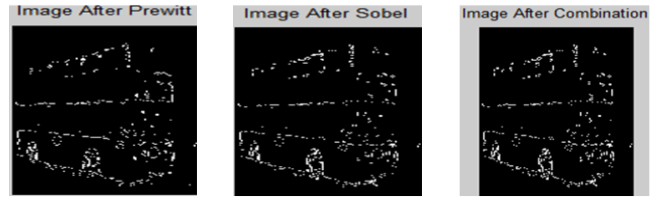
Figure 6. Edge Detection Results on Bus Image
