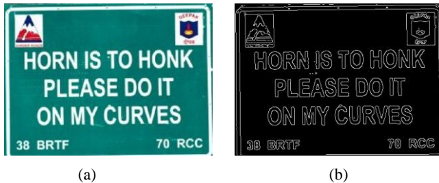
Figure 2. (a) Input JPEG image (b) Edge image after applying canny edge detection algorithm
