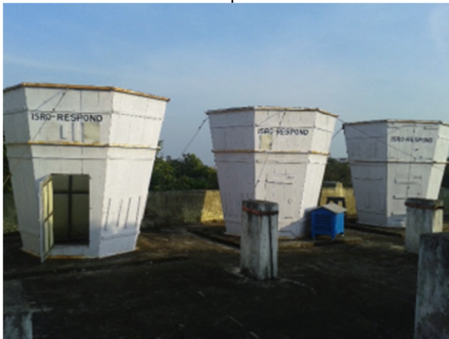
Figure.3: SODAR antenna at Dept. of Systems Design, Andhra University. Sponsored by UGC and ISRO
