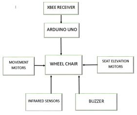
Fig 4: Wheelchair Block Diagram.
