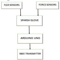
Fig. 1: The Sparsh Glove Block Diagram
