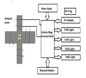
Density of vehicle is higher on lane then controller set max time of signal. An emergency vehicle is detected then controller set time of signal and change light of signal.
