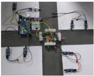
This is a snap of our actual working model. The IR sensors monitor the density and Arduino board is our microcontroller
