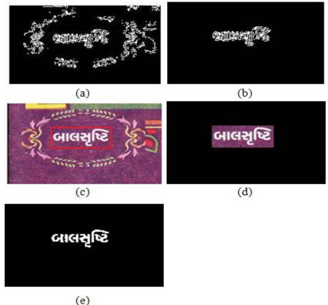
Figure 6. CC analysis (a) connected component (b) candidate text area after filter out non-text regions (c) Detected text region marked by red rectangle(d) isolated text region (e) Binary of detected text
