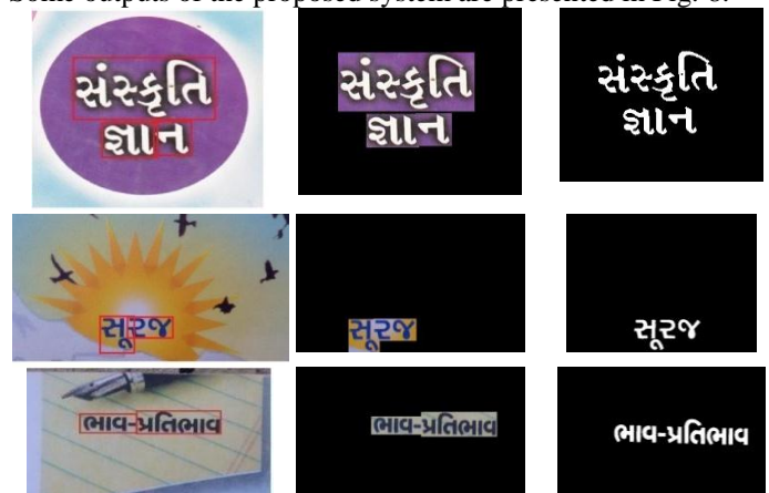
Figure 7. Image has text of both polarity (a) detected text (b) text binarization before text polarity step (c) text binarization after text polarity step
