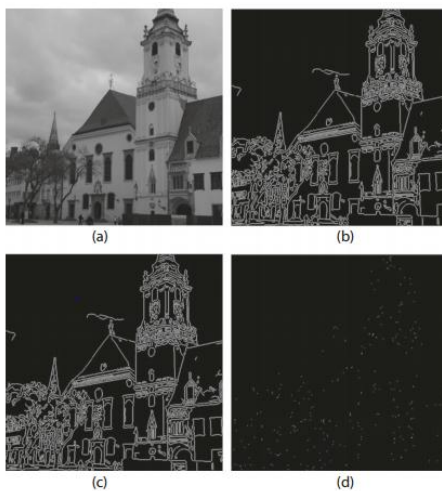
Figure 1.2: (a) cover image (b) cover image edges (c) stego image edges (d) difference between cover image edges and stego image edges [3].
