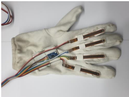
Figure 9a: Normal gloves converted to smart data gloves
