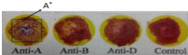
Figure 2: Fabric test strip appearing of blood for member T3 with blood classification AB+. Note that agglutination is available in the initial three circles while the control remains un-agglutinated. Likewise demonstrated is the recorded square picture A* portrayed in Section II.D.
