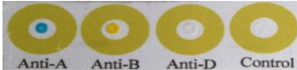
Figure 1: Fabric based test strips. At the focal point of each yellow circle, silk yarn covered with antibodies relating to A, B and Rh are available. The Control circle does not have any antibodies present at its middle.
