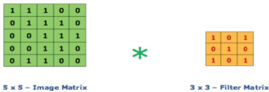
Fig.3.1.5. Image matrix multiplies kernel or filter matrix
