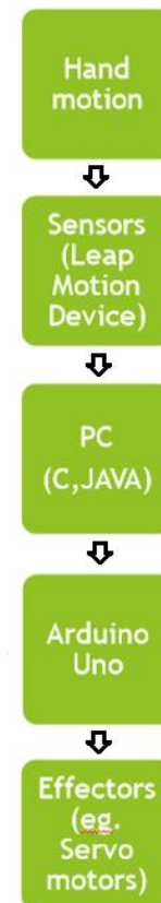
Figure 1. Flowchart for controlling a robotic arm using leap motion
