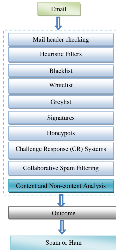
Figure 6. On applying different filtering techniques to incoming email, outcome is either spam or ham
