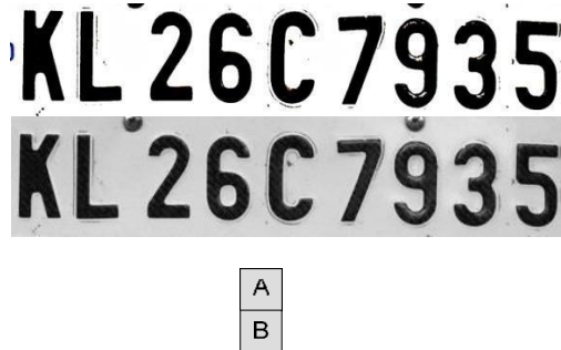
Figure 10 The input a and output b example of segmentation phase of the ANPR recognition process.
