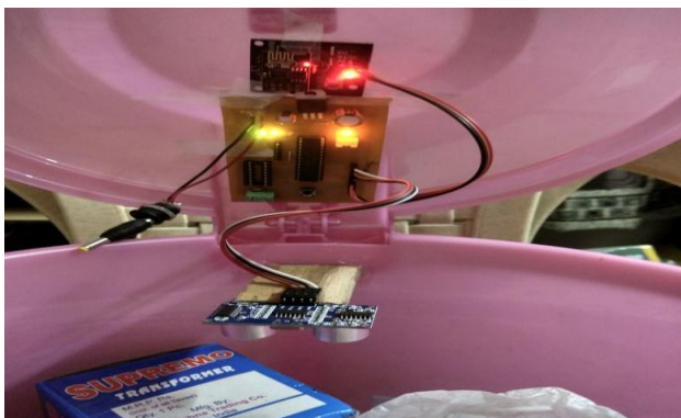
Figure 4. Yellow LED is on when bin is filled
