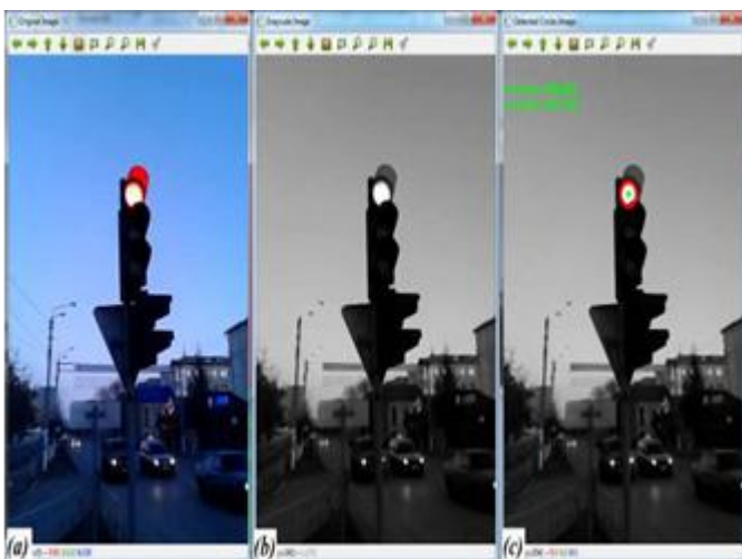
Fig-2: (a) Traffic light color image. (b) Gray scale image. (c) Cropped traffic signal image. Convolution
