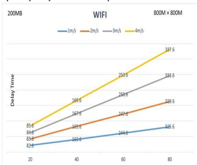
Fig. 6 Performance of Wi-Fi handover results for 200 MB in 800m × 800m
