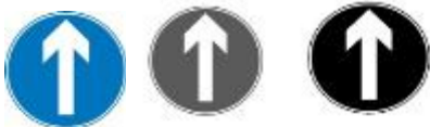
Fig.2 The road symbol has been detected: The given symbol is converted to gray scale and then the blue frames are subtracted to get the binary image.
