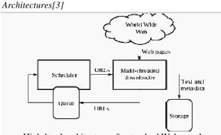
High-level architecture of a standard Web crawler
